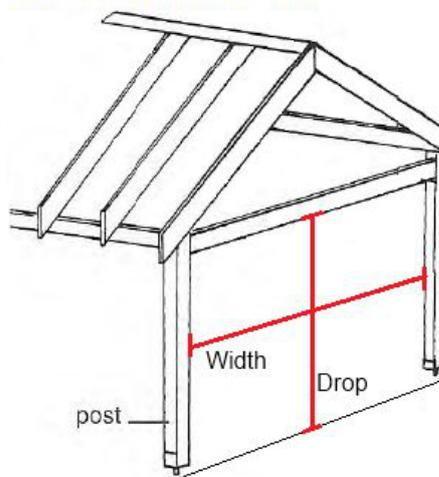
**NOTE:** We recommend measuring each opening in 3 different positions for the width and the drop. For the width - measure the top, centre, and bottom, and for the drop - measure left, centre and right.
